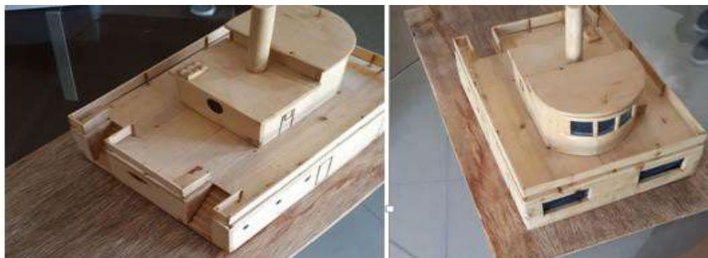
Figure 24: Finished Superstructure. Source: Autorers,2021
