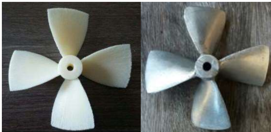
Figure 9: 3D Printed Model and After Casting. Source: Authors,2022
